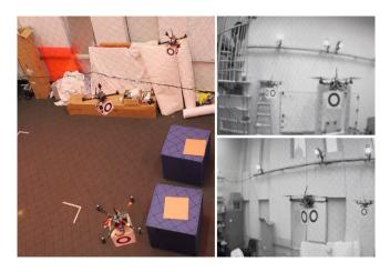
Fig. 1. Decentralized formation flight based on relative localization performed by the presented method. Courtesy of the GRASP laboratory, IJPENN
