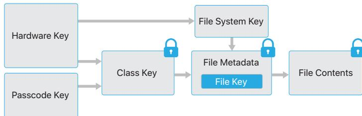
The content of a file may be encrypted with one or more per-file (or per-extent) keys that are wrapped with a class key and stored in a file’s metadata, which in turn is encrypted with the file system key. The class key is protected with the hardware UID and, for some classes, the user’s passcode. This hierarchy provides both flexibility and performance. For example, changing a file’s class only requires rewrapping its per-file key, and a change of passcode just rewraps the class key.
