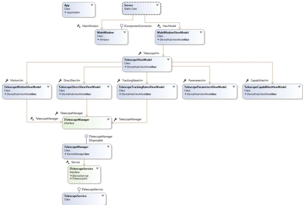
Unfortunately, the Visual Studio class diagram tool does not provide the ability to define the dependency between the App class and the static Server class. The best that I can do is to simply show the App class. The dependency does exist, however. The App’s instance overrides the base class’ OnStartup method to invoke the Server class Startup method and pass it any command-line parameters.
