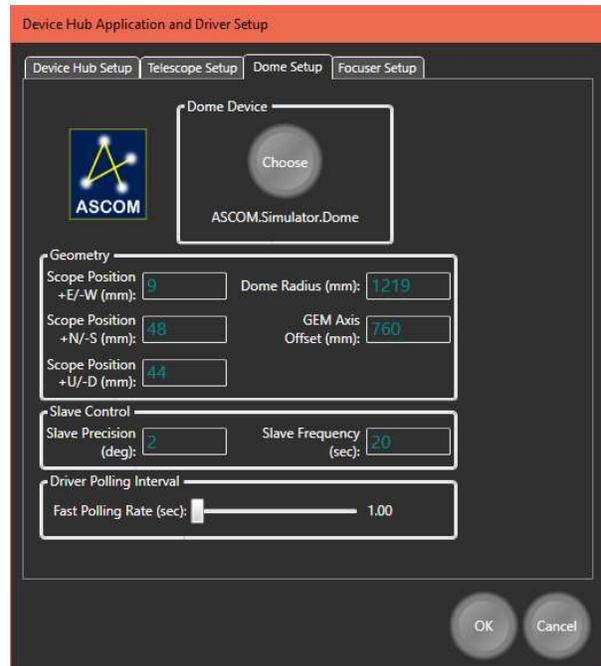
Other Dome configuration settings include the radius of the dome, the distance from the intersection of the RA and DEC axes (Point A) to the nearest point along the centerline of the telescope's optical path. This is the GEM Axis Offset value (760 mm) in the screenshot. It should be 0 for a non-GEM mount.
