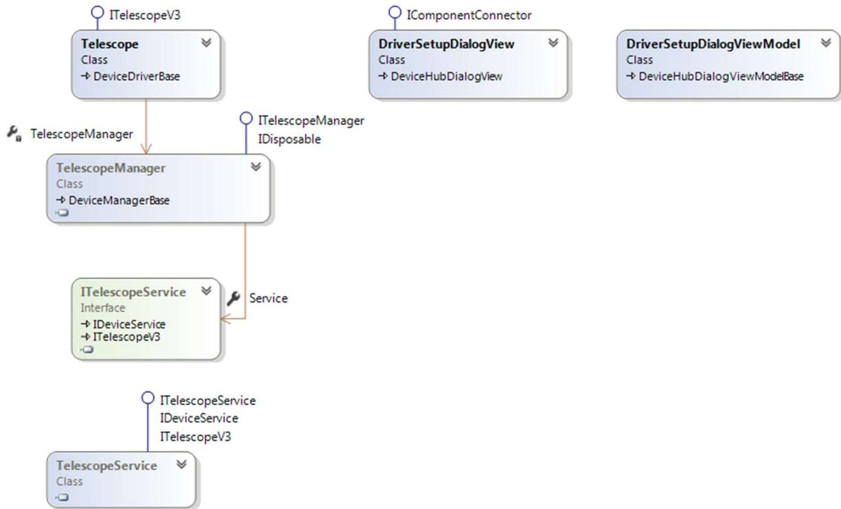
The Telescope driver implements the ITelescopeV3 interface and derives from DeviceDriverBase which derives from ReferenceCountedObject. DeviceDriverBase provides convenience methods that are used for data and state validation by the device drivers. It also provides common methods for logging.
