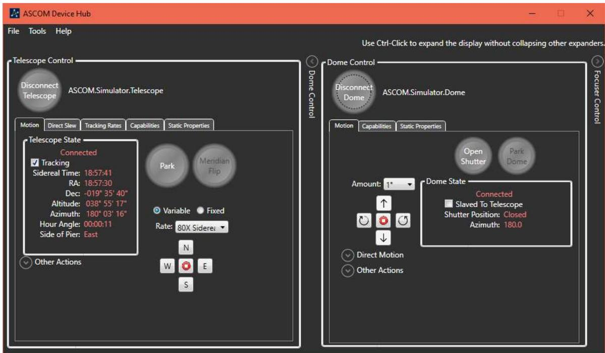
The next configuration setting allows you to choose to keep the Device Hub user interface windows as the topmost windows on the display. When this setting is changed, you must shut down and restart Device Hub for the change to be recognized.
