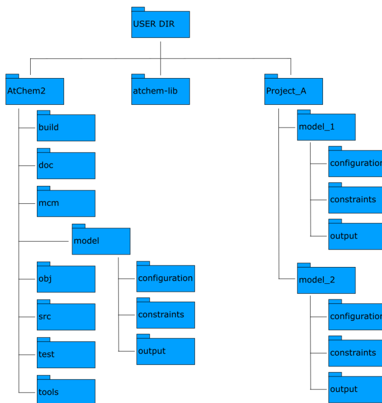
Figure 4.1: Example of a modelling setup, with an AtChem2 installation and a project directory containing two box-models.
