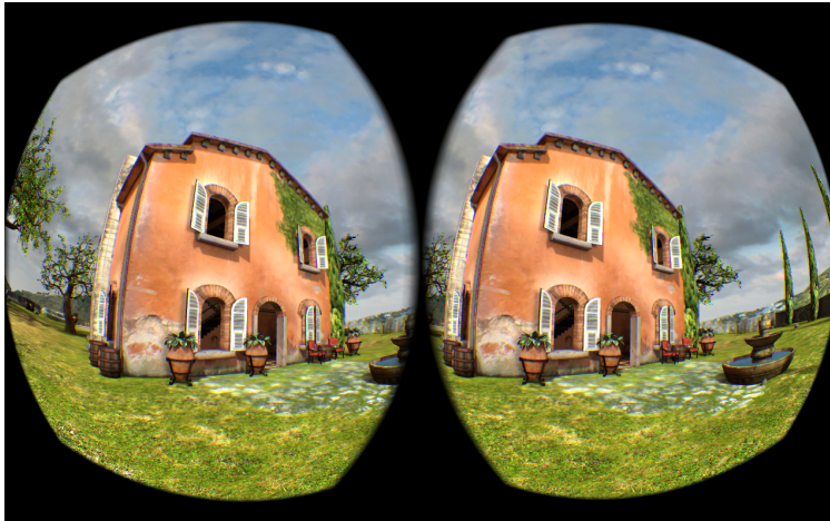
Figure 8: OculusWorldDemo stereo rendering.
