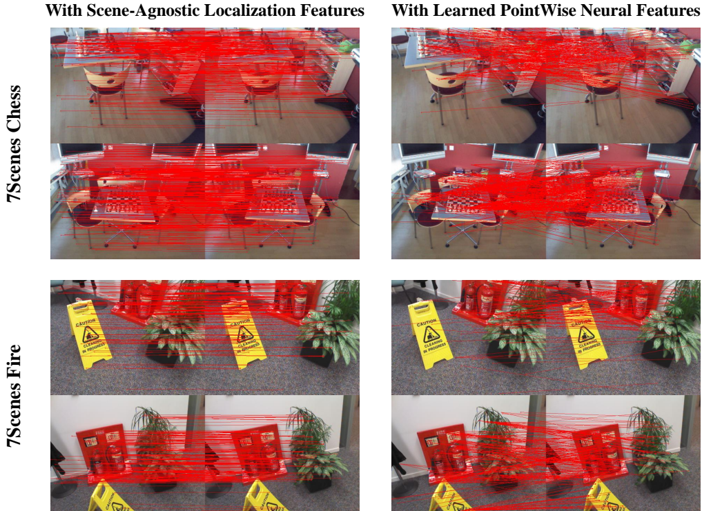
Figure B: Feature matching results. We compared the matching results with different features. Specifically, we extract 800 key points from the query image. The features extracted on the left images are scene-agnostic localization features, while those on the right are learned pointwise neural features. We then match 2D key points with the 3D points in the point cloud by computing the cosine similarity and project the corresponding 3D points onto the query image using the ground truth camera poses. Finally, we illustrate the matching relationships and demonstrate the necessity of using a localization feature extractor instead of the learned pointwise neural features for feature matching.
