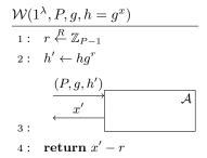
Figure 2: The toy version of random self-reduction for discrete log that randomizes only h.
