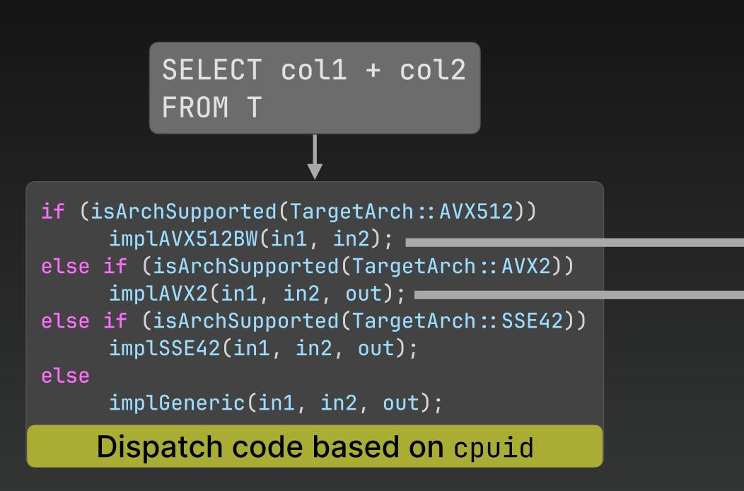
• The fastest kernel is selected at runtime based on the system capabilities (cpuid).
