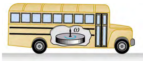
FIGURE 10.15 Experimental vehicles, such as this bus, have been constructed in which rotational kinetic energy is stored in a large flywheel. When the bus goes down a hill, its transmission converts its gravitational potential energy into KE_{\text{rot}} . It can also convert translational kinetic energy, when the bus stops, into KE_{\text{rot}} . The flywheel's energy can then be used to accelerate, to go up another hill, or to keep the bus from slowing down due to friction.
