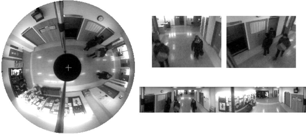
Figure 2: The OmniVideo system. A panoramic view and multiple perspective views (right) are created from a single omnidirectional video frame (left).
