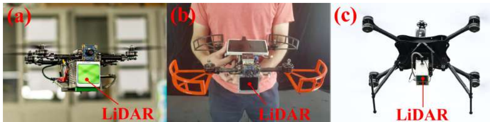
Figure 3.5: Three different platforms: (a) 280 mm wheelbase small scale quadrotor UAV carrying a forward-looking Livox Avia LiDAR, (b) handheld platforms, (c) 750 mm wheelbase quadrotor UAV carrying a down-facing Livox Avia LiDAR. All three platforms carry the same DJI Manifold-2C onboard computer. The video of real-world experiments is available at https://youtu.be/20vjGnxszf8 .
