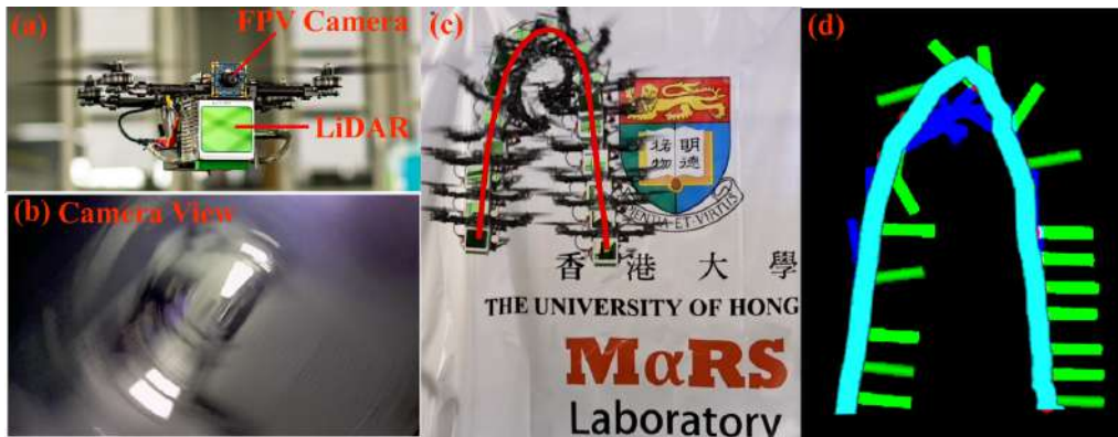
Figure 3.8: The flip experiment. (a) the small scale UAV; (b) the onboard camera showing first person view (FPV) images during the flip; (c) the third person view images of the UAV during the flip; (d) the estimated UAV pose with FAST-LIO2.
