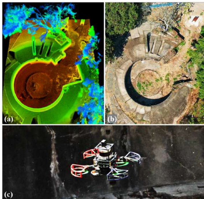
Figure 4.18: Our proposed framework D-Map served as a real-time high-resolution occupancy mapping module for an autonomous UAV exploration task in an ancient fortress. (a) The high-fidelity point cloud collected by UAV. (b) A bird-view of the scene. (c) The aerial platform carried a 128-channel LiDAR (OS1-128) to conduct the exploration task. The accompanying video of this paper is available on Youtube: youtu.be/m5QQPbkYYnA .
