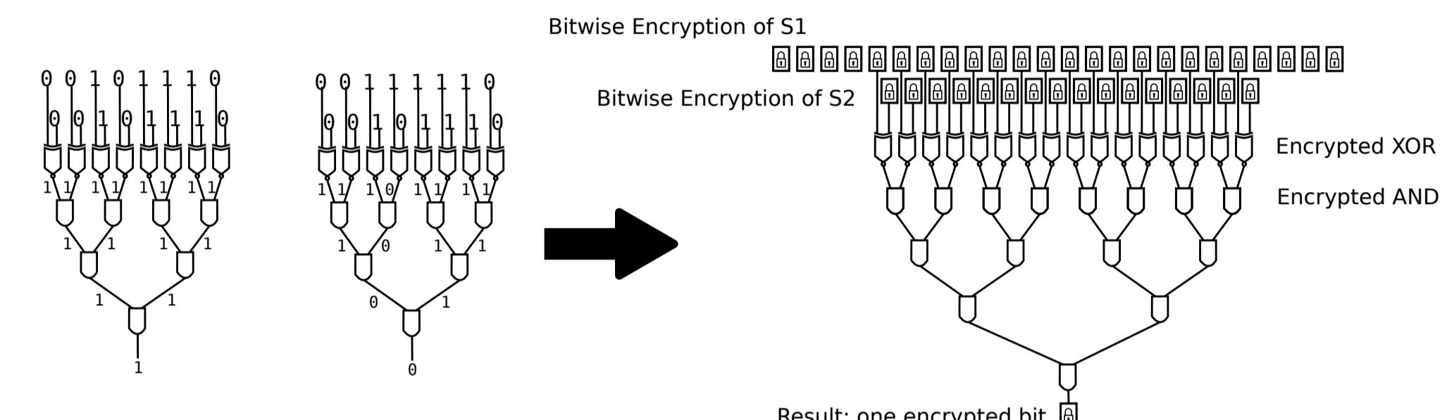
When comparing 8-bit characters with Boolean circuits, the result is 1 when the characters are equal and 0 when they are unequal
