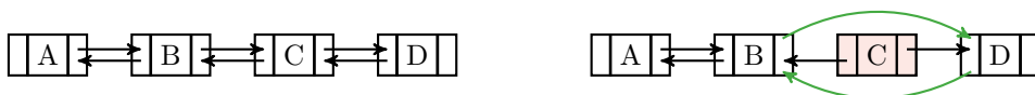
Figure 1.4: Removal for doubly linked Lists. To avoid gaps in the chain, nodes B and D must be linked together. Python will automatically delete node C since there are no references to it.
