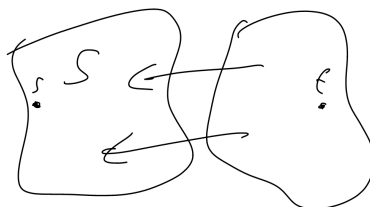
Figure 11.1: Example of a cut: No edges go from S to (S, V \setminus S) , and so the value of this cut is zero.
