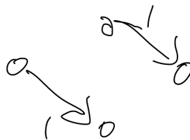
Figure 11.4: Remaining edge capacities after sending a path flow through the graph as depicted in Figure 11.3.
