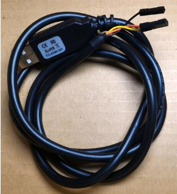
**Figure 13-3.** USB to UART cable—TTL-232R-3V3/TTL-232R-RPI
