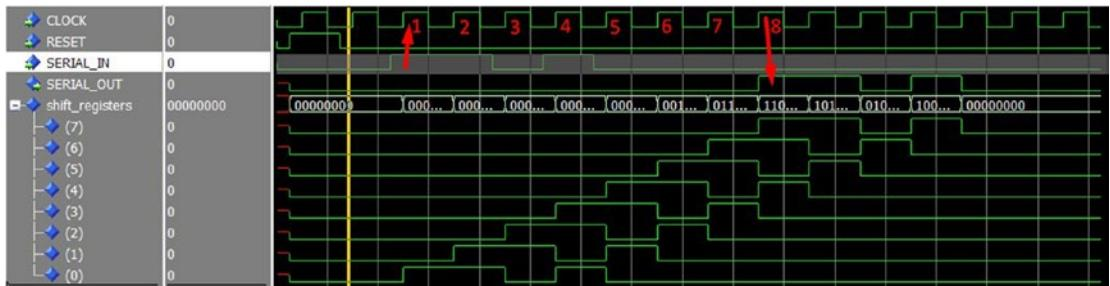
**Figure 10-6.** Simulation result for 8-bit SISO Shift register
