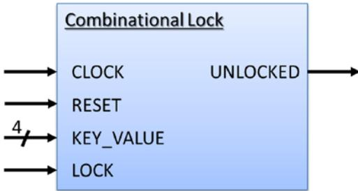
**Figure 11-8.** *Combinational lock block diagram (inputs and output)*
