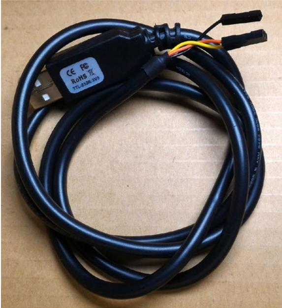
**Figure 13-3.** USB to UART cable—TTL-232R-3V3/TTL-232R-RPI
