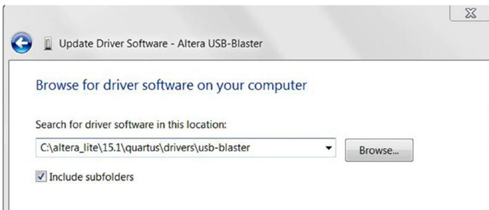
**Figure 4-54.** Update Driver Software - Altera USB-Blaster
