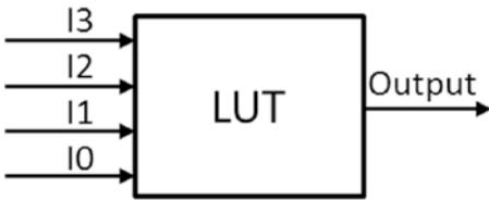
Figure 1-3. Four inputs, one output Boolean function
