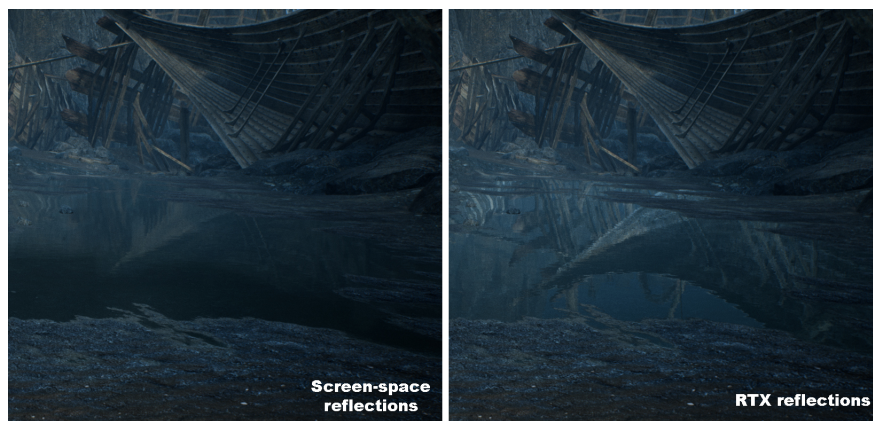
FIGURE 3.12: Screen-space reflections (left) vs ray-traced reflections (right). Screen-space reflections are generally less resource-intensive, but can only reflect geometry that is rendered to the screen itself. Images taken from the PC game Hellblade: Senua's Sacrifice by Ninja Theory .
