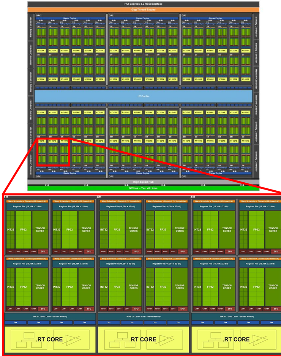
FIGURE 3.2: Architecture of the TU102: 6 GPCs, each consisting of 6 TPCs that contain 2 SMs each. Each SM contains a number of ALUs for integer, floating point and matrix operations as well as a single RT core. Each RT core has a separate core for BVH traversal and triangle intersections respectively. Image adapted from the Turing architecture whitepaper [49].
