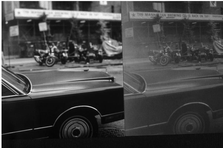
FIGURE 2.2: Normal lens (left) vs. Pinhole lens (right). The pinhole has greater depth of field, but the image sharpness decreases with pinhole size. Image credited to Leonard Lessin/Science Source [60].
