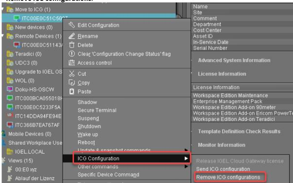
The endpoint device is removed from the ICG.
