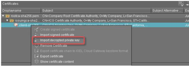
(i) If the private key is protected with a passphrase, you need to decrypt it using the OpenSSL command line tool: openssl rsa -in encrypted.key -out decrypted.key
