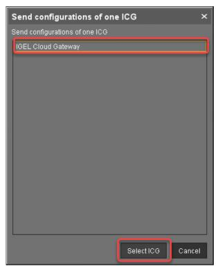
If everything went well, the devices connect to the specified ICG. If the ICG is not reachable at this moment, the ICG configuration remains unchanged, and the devices stay connected to the local UMS network or to the old ICG.
