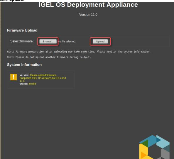
The upload process starts. When the upload is finished, the Deployment Appliance starts to prepare the firmware.
