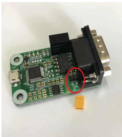
Disable 120 Ohm Resistor
