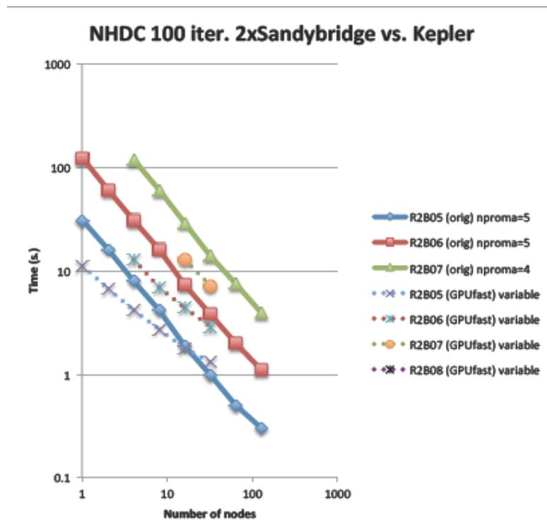
Figure 20 - Compare original (GNU) on Cray XC30 (2x Sandybridge sockets) vs. XK7 node with Kepler K20x (Cray CCE)
