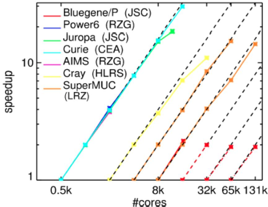
Figure 26 – VERTEX performance on main HPC architectures
