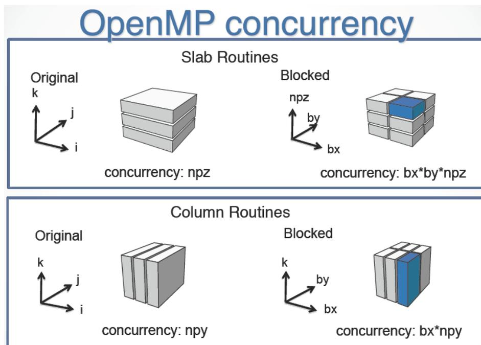
Figure 12 – Slab and column concurrency approaches
