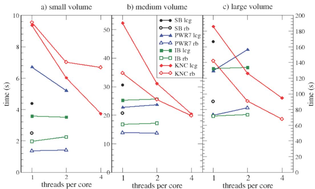
Figure 9 – Performance comparison among Xeon Phi and Intel processors
