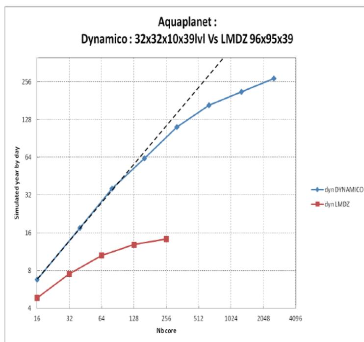
Figure 6 - Performance comparison between DYNAMICO and LMD-Z
