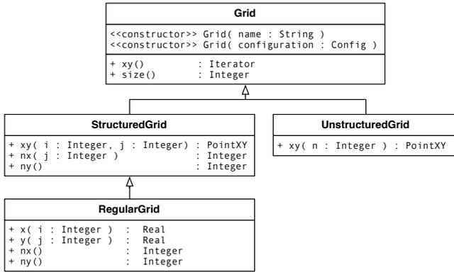
**Figure 4.** Object orientation and the *Grid* classes supported in Atlas. Specific model grids can be constructed as instances of one of these classes. For example, the current ECMWF high resolution (9km) octahedral reduced Gaussian grid is an instance of the StructuredGrid, but can be referred to by the name Ø1280 which it inherits from the Grid class.
