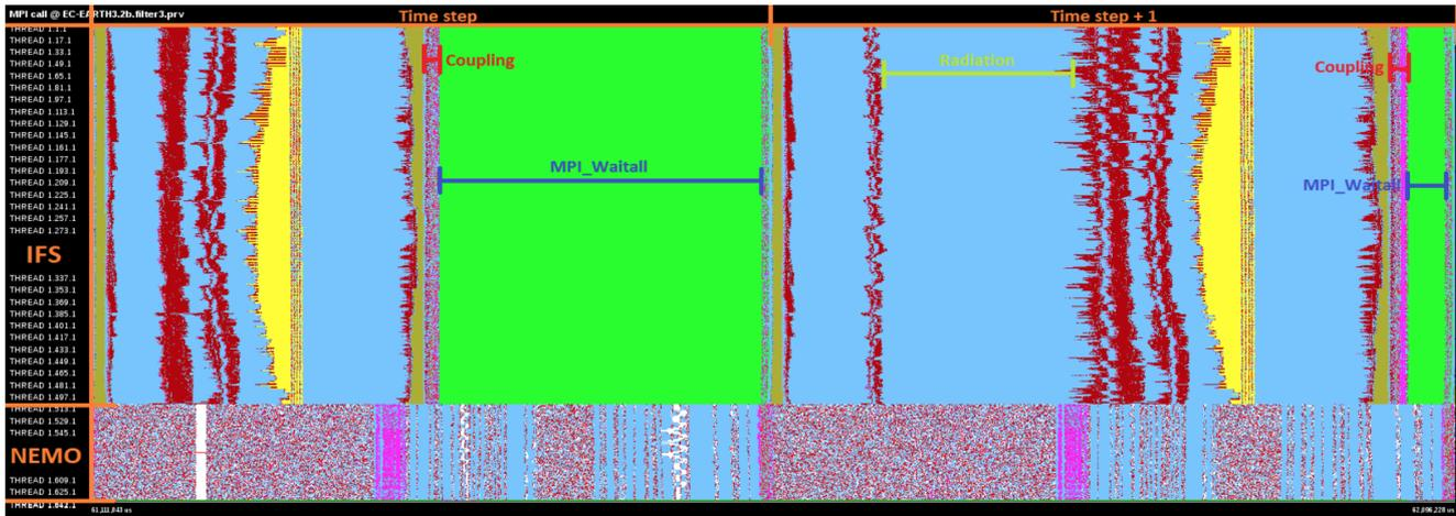
**Figure 8.** Example trace information generated with EXTRAЕ used to analyse high resolution coupling in EC-Earth. This view shows MPI calls during the execution (one color per call). On top, 512 MPI tasks for IFS atmospheric model and bottom, 128 MPI tasks for NEMO ocean model. This fine-grained performance information yields information as to how to get better performance out of coarse grained concurrency.
