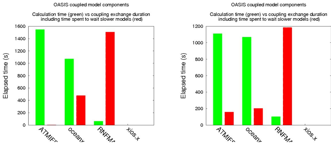
Figure 3-a & 3-b: Load balancing analysis of EC-Earth coupled system with different parallel decomposition of IFS (256 & 512) and the same decomposition of NEMO (128)
