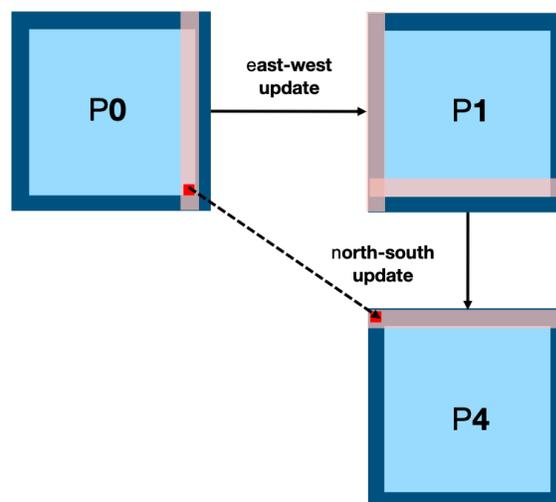
Figure 2 - NEMO LBC update. In the picture we assume to have a 3x3 grid of processes.
