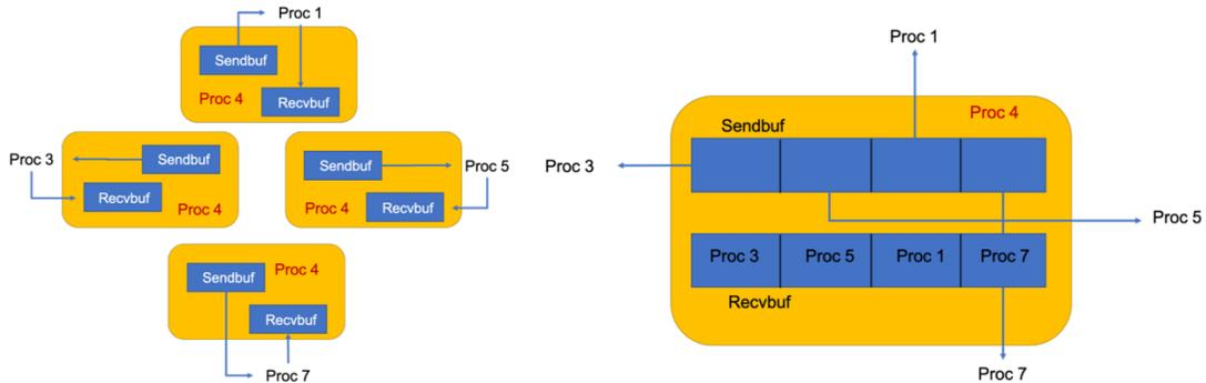
Figure 4 - MPI messages exchanged with current P2P communications (left side) and MPI3 neighbourhood collectives (right side)
