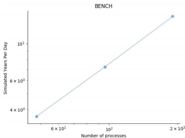
Figure 1: Scalability of nemo model with BENCH
