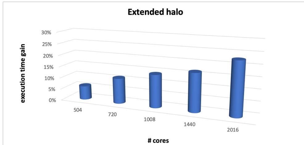
Figure 10 - Execution time improvement (%) of extended halo version compared with original one
