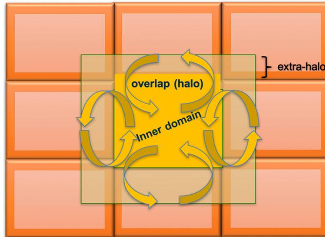
Figure 9 - Extended halo exchange
