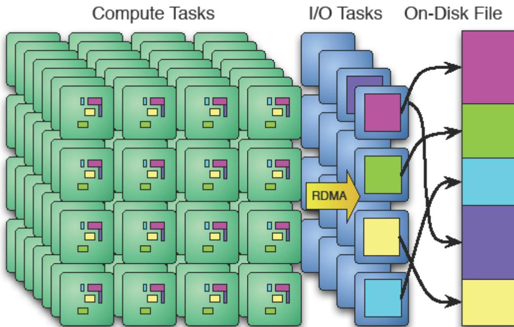
Figure 11: Data transfer in a parallel program employing CDI-pio I/O server tasks for output. The data decomposed into small chunks on the compute tasks is gathered by variable on I/O tasks with one task gathering one or more variables. All I/O then collectively write to the resulting on-disk file.
