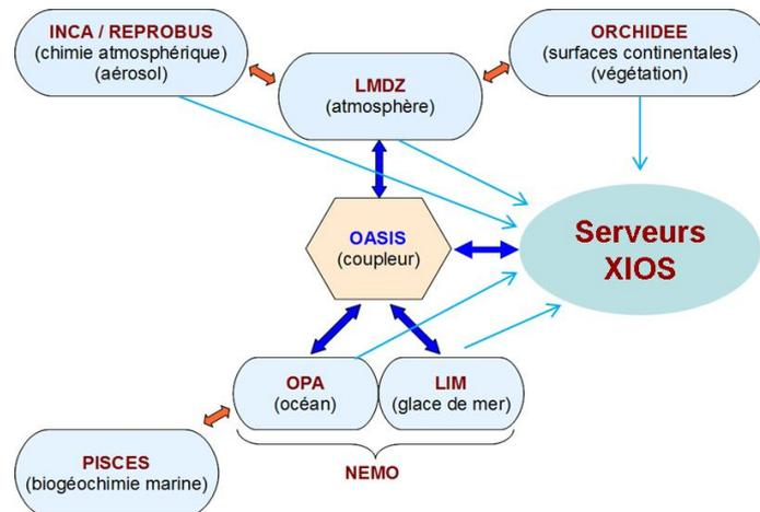
Figure 6 : interaction between the XIOS library, the OASIS coupler and the component models in the IPSL Earth system model.
