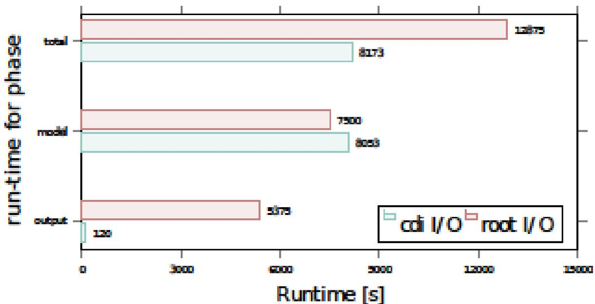
Figure 12: Employing parallel I/O via CDI-pio significantly reduces total run-time by virtue of almost complete elimination of waiting on I/O as previously witnessed for single-task root I/O for ECHAM6 (see text for specifics of configuration)
