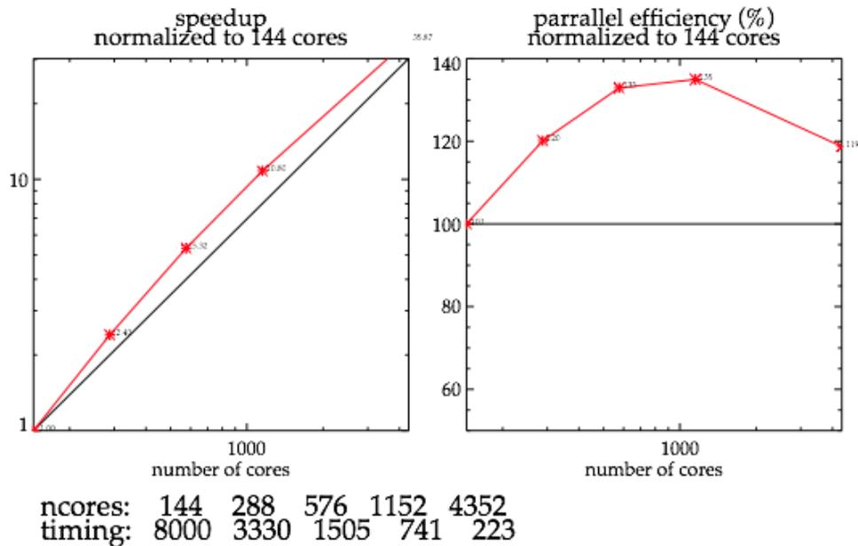
Figure 10 : Performance data obtained on the Curie supercomputer
