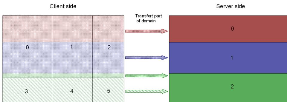
Figure 7 : data distribution between model domains of clients and servers. On the client side, data distribution is driven by the model and, on the server side, the distribution is driven by optimal disk operation, i.e. are evenly distributed and memory contiguous.
