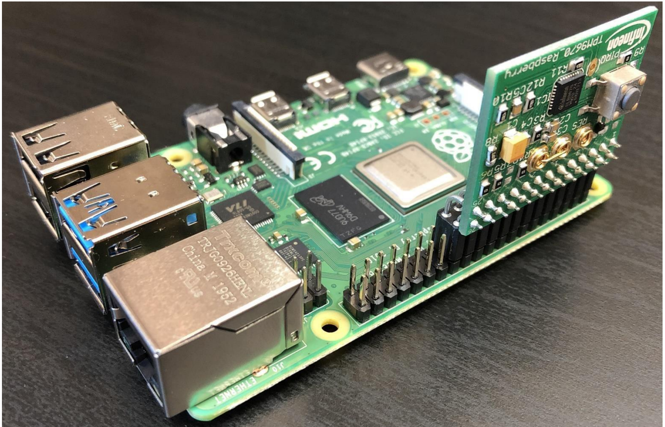
Figure 1 Infineon Iridium SLx 9670 TPM2.0 SPI Board on Raspberry Pi® 4
