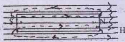
(b) Paramagnetic substance in a magnetic field
