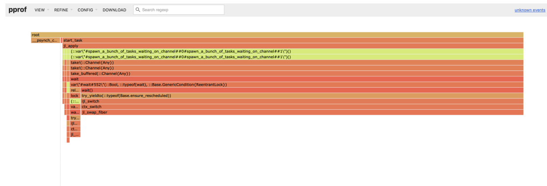
Figure 33.2: Wall-time Profile Channel
