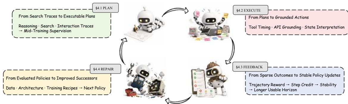
Figure 4: Where model-side interventions enter the plan–execute–feedback–repair loop. Planning turns successful traces into training examples for future plans. Execution trains the model to choose tools and interpret returned state. Feedback assigns outcomes to the actions that caused them. Repair changes the data, architecture, or training recipe used to produce a successor policy. Arrows mark functional roles, not a fixed chronology.
