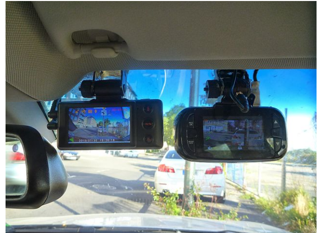
Figure 1. Dashcam installation on the front windshield [1]
