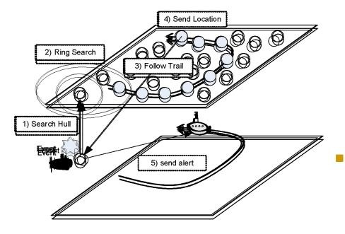
A mobile node first routes a query packet vertically upwards to the node on the projected position of the convex hull plane Node performs an expanding spiral curve search to find a pheromone trail.
