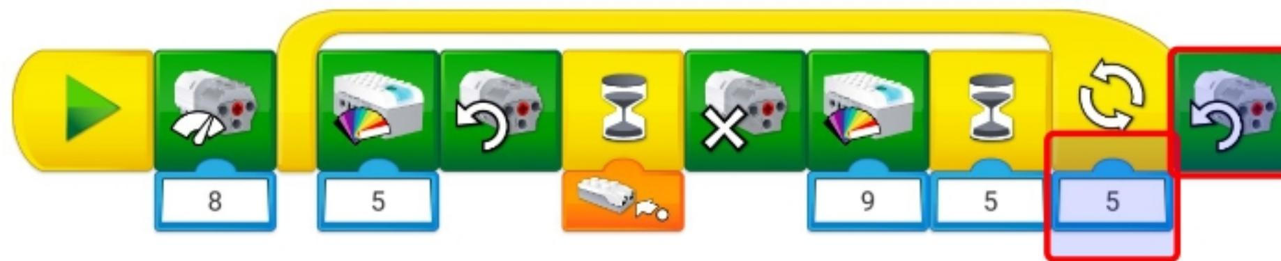
With such settings, the loop repeats the blocks placed in it five times, after which the next block will run the motor.
