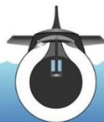
For pop up the tanks must be filled by air. In this case the submarine's average density is less than the water's.
