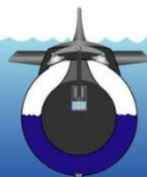
In this case the submarine's average density is equal to the water's.
