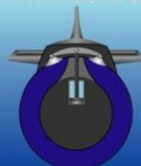
For the dive the tanks must be filled by the water. In this case the submarine's average density is more than the water's.
