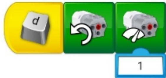
In order to control the manipulator more precisely, it is convenient to use a low speed. In our case - "1".
