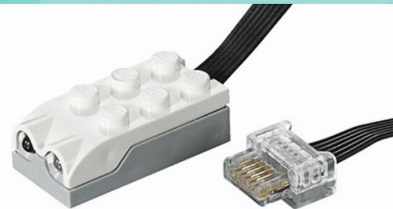
The sensor emits infrared light (like a TV remote or conditioner) and measures the amount of light returned. If a lot of light has returned, then the object is nearby, and if it is small, then the object is far away.
