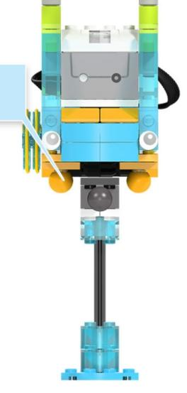
Note, that Guides not touches the rail on the straight sections. But they works on the curves.
