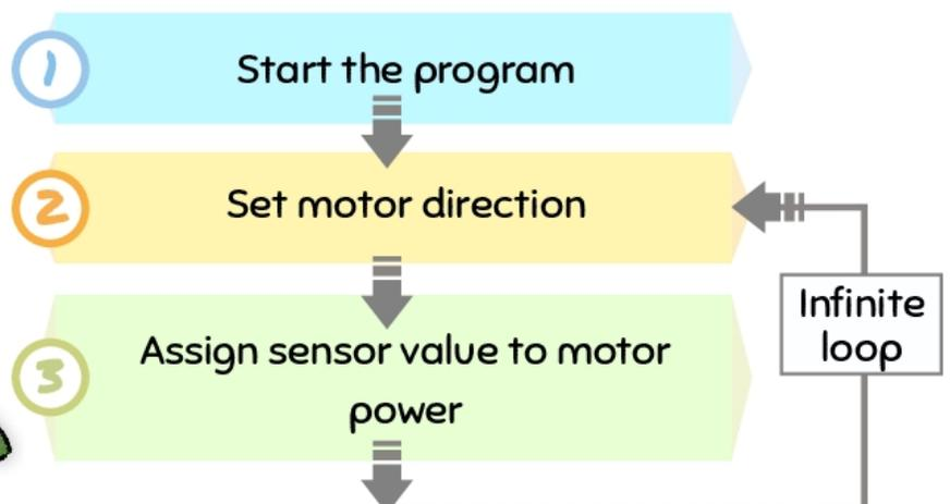
• The flowchart indicates **three tasks**. Therefore, you can assign a **programming block** for **each task**:
