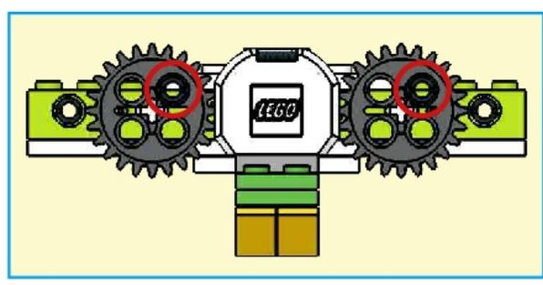
**Be careful!** The pelican uses an “in-phase” motion, meaning that one of the axles is in the exact same position of the other one.
