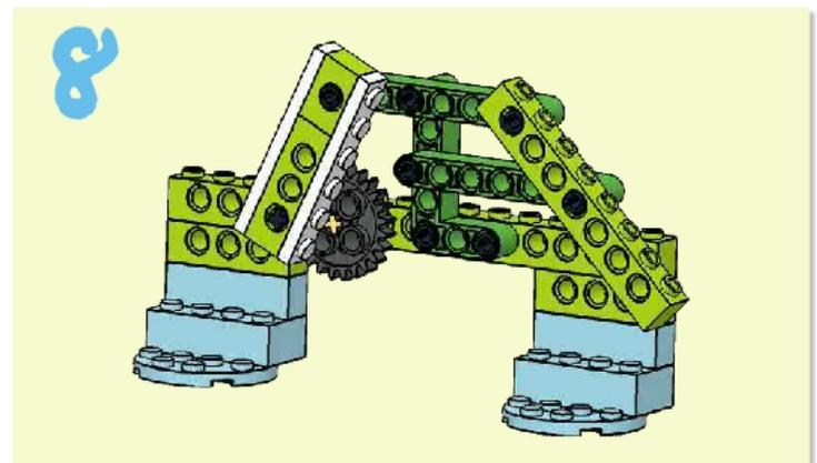
• Spin the gear to see the generated **flapping wings motion**.
