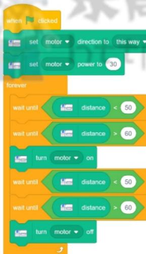
The robot starts moving and stops after detecting a wave of the hand
