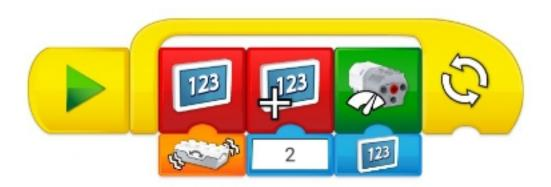
In the horizontal position sensor displays a "O". Therefore, the rotors did not turn. If you add a small number to the sensor, for example, 2, the rotors will not stop, and at different positions of the robot, the rotors will have different speeds.
