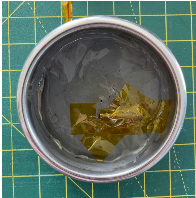
Figure 11: Thermofilter basket with thermofilter taped in place. 1/2 inch scale.
