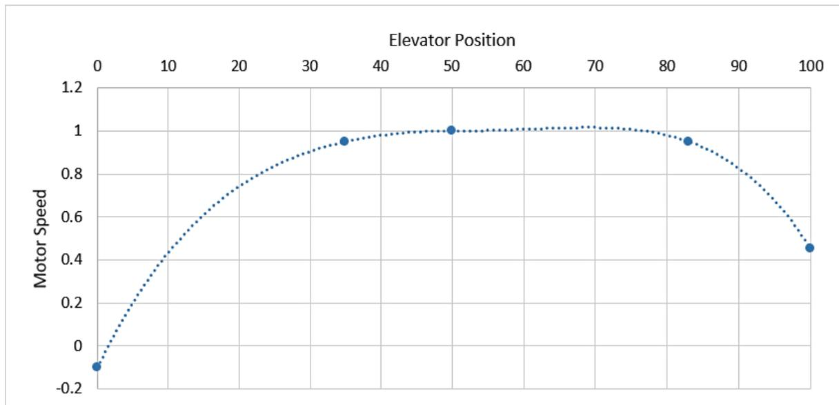
The elevator subsystem now includes a “throttled” function, that automatically adjusts the speed of the elevator depending on the position.
