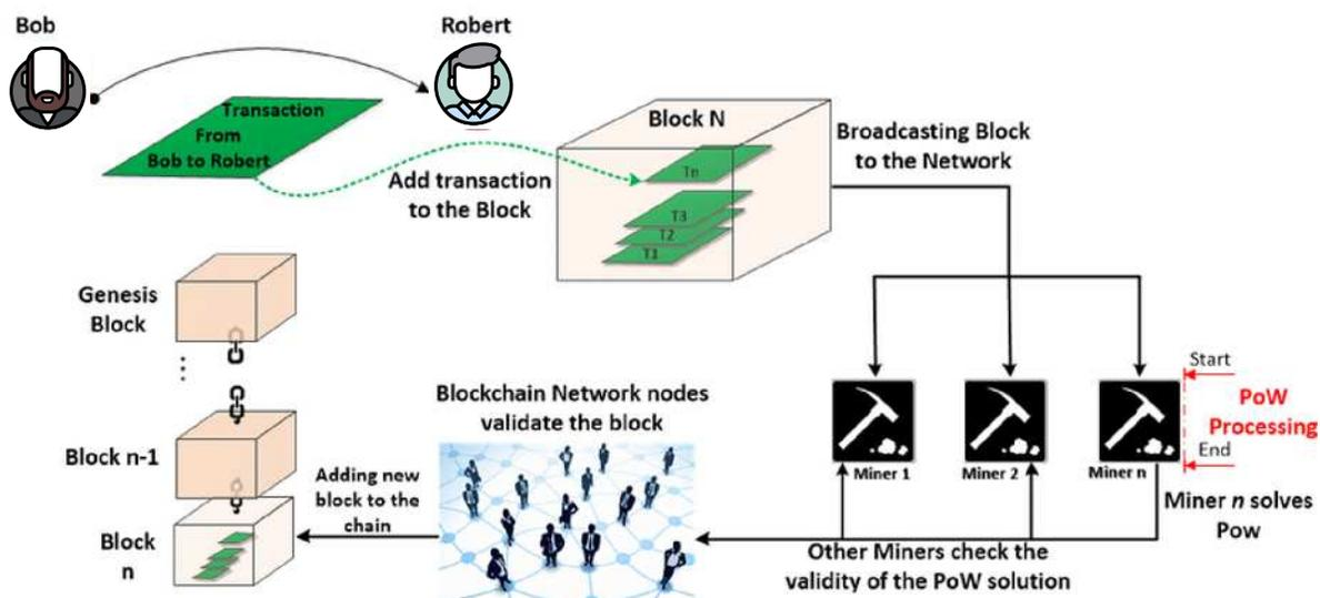
4. The nodes verify the **transaction** using the sender's **public key**, which is available on the **blockchain**. They check that the signature is valid and that the sender has enough **bitcoin** to complete the **transaction**.
