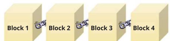
The blocks are “linked” together by enforcing a specific relationship between blocks. That is, a block must contain a “fingerprint”, which is a hash value of the data of the previous block. A hash function can condense arbitrary message (the block information) to a fixed size (e.g., 160 bits) and produces a fingerprint of the message.
