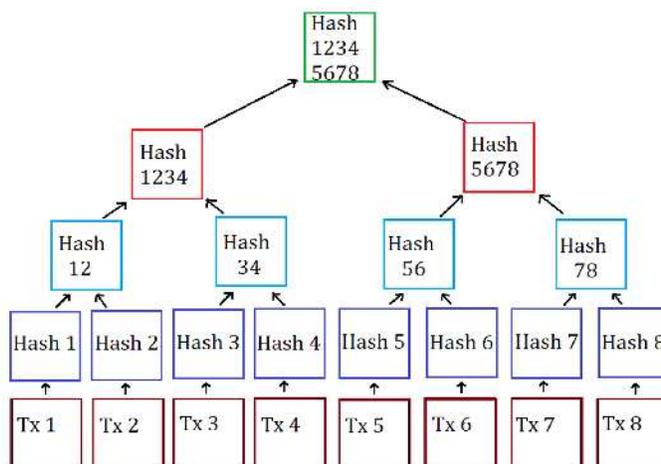
The **Merkle Root Hash**, which is the data included in the header, is a **single hash value** that acts as a digital fingerprint for all the transactions in a block. This allows for efficient verification of transactions without having to examine each one individually, making it an important component of the security and scalability of the Bitcoin network.
