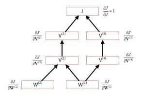
Figure 2.6: An efficient gradient computation algorithm in CN.  $\mathbf{W}^{(1)}$  and  $\mathbf{W}^{(2)}$  are model parameters. Each node n stores both the value of the node  $v_n$  and the gradient  $\nabla_n^J$ .
