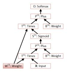
Figure 2.3: A computational network with shared model parameters (highlighted). Here we assume the input  $\mathbf{X}$ , hidden layer  $\mathbf{S}^{(1)}$ , and output layer  $\mathbf{O}$  have the same dimension.
