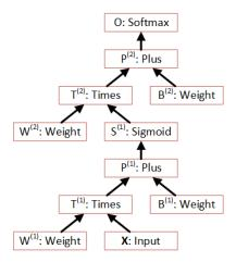
Figure 2.1: Represent the one-hidden-layer sigmoid neural network of Algorithm 2.1 with a computational network
