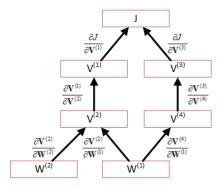
Figure 2.5: The naive gradient computation in CN.  $\mathbf{W}^{(1)}$  and  $\mathbf{W}^{(2)}$  are model parameters and each edge is associated with a partial derivative.
