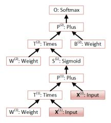
Figure 2.2: A computational network with two input nodes (highlighted).
