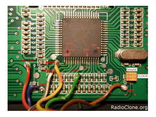
Once the oscillator is connected, you simply connect the 9X to your programmer as you normally would. The oscillator will be powered through the programmer, and will output a 1MHz oscillator signal to the ATMEGA64, and you will be able to access your radio again to reprogram it.
