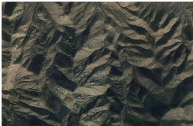
Figure 1: RGB image for the NEON Santa Rita Experimental Range (SRER) site. Differences in terrain orientation could cause variations in the reflectance values between pixels with similar land cover types and canopy structural properties (Image Source: Google Maps).
