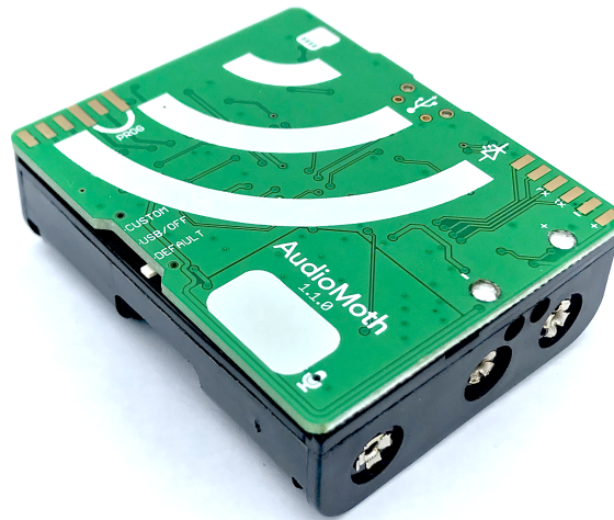
Figure 1: AudioMoth 1.1.0: A low-cost, low-power acoustic monitoring device developed for a wide variety of conservation projects.
