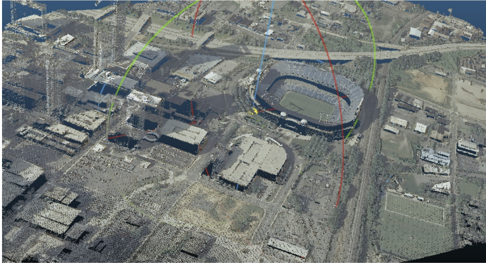
Fig. 5: After colorization, points take on the colors provided by the input image
