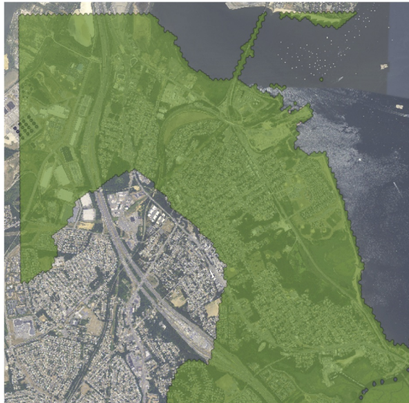
Fig. 8: Hexbin output shows boundary of actual points in point buffer, not just rectangular extents.
