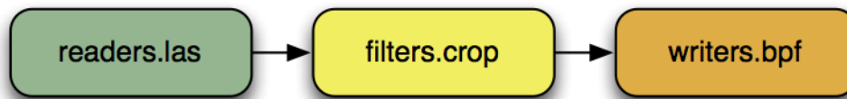
Fig. 1: A simple pipeline to convert LAS (page 79) to BPF (page 57) while only keeping points inside the box [0 \leq x \leq 100, 0 \leq y \leq 100] .
