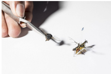
Figure 1: Profile of a typical micromechanical flying insect[3]
