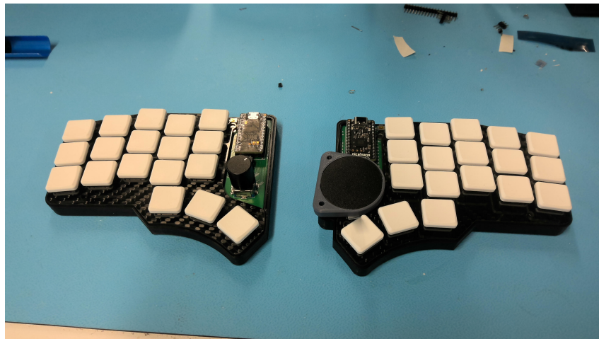
Figure 29: Daedalus just after finished soldering and fitted inside the temporary casing
