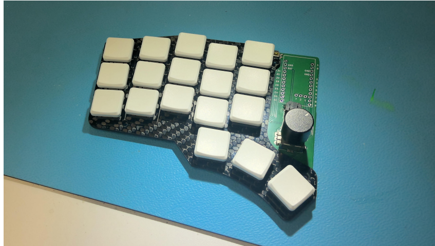
Figure 22: Keys soldered to the PCB with the carbon fiber plate in between
