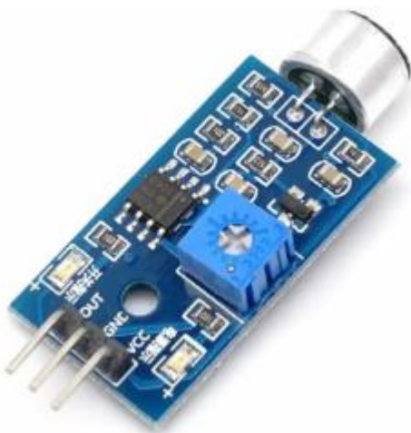
Sound sensor – Pulses signal high when sound is detected
