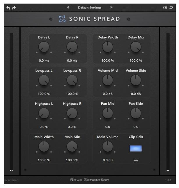
Delay L (ms): Adjusts the delay time for the left channel, from 0.0 ms to 40.0 ms.
